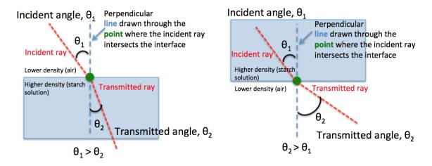
An equation that relates the incident angle  $(\theta_1)$  and transmitted angle  $(\theta_2)$  of the light beam to the different speeds of light  $(v_1 \text{ and } v_2)$  in media of two different densities is called Snell's Law:
